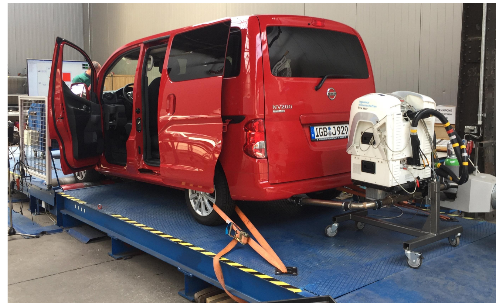
2: Fix the car on a chassis dynamometer, attach an emissions measurement device, calibrate it, ...
